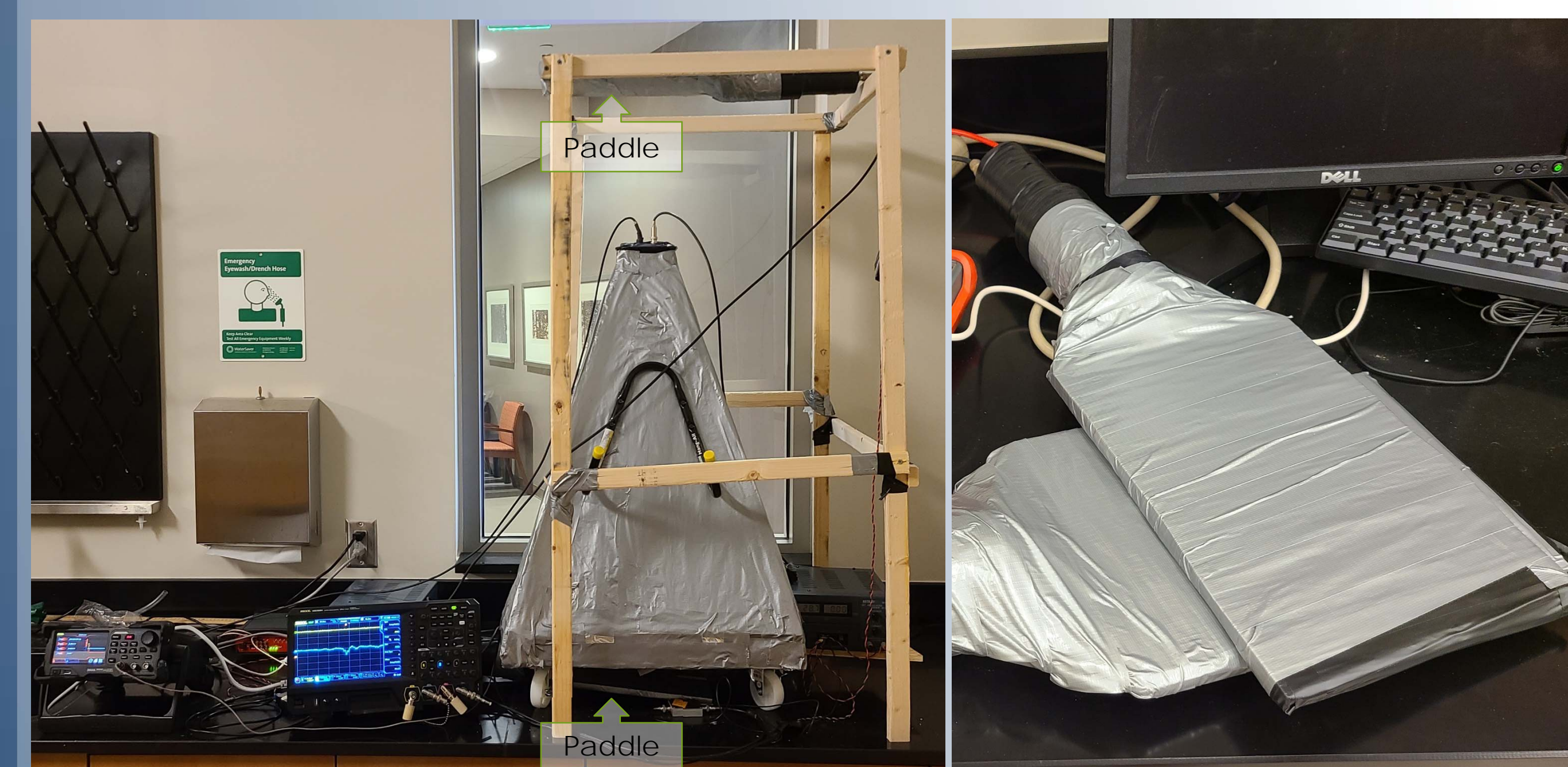
Figure 4: (left) DUCK system prototype module connected to an oscilloscope and power supplies. The triggering paddles forming a hodoscope are at the top and bottom of the module. (right) Triggering paddles.
